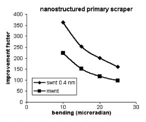
Fig. 4. The same data as in previous figure, plotted as an LHC background reduction factor 1/(1 - F) as a function of bending angle, for carbon SWNT and MWNT.
