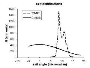
Fig. 2. Angular distributions downstream of a primary target due to elastic nuclear scattering on the atoms of amorphous carbon target and due to channeling in carbon SWNT target.
