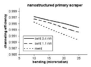
Fig. 3. The overall (multi-pass) channeling efficiency *F* of nanostructured scraper shown as a function of bending angle for SWNT (0.4 and 1.1 nm diameter) and MWNT at 7 TeV.
